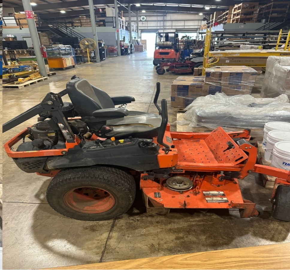
Mower #4 Kubota Z725 60" Cut; Motor: 801V KW; Machine Hours: 1,520; Fair Condition; Works as it should; Needs oil change, needs pulleys and bearings; SN: 14326
