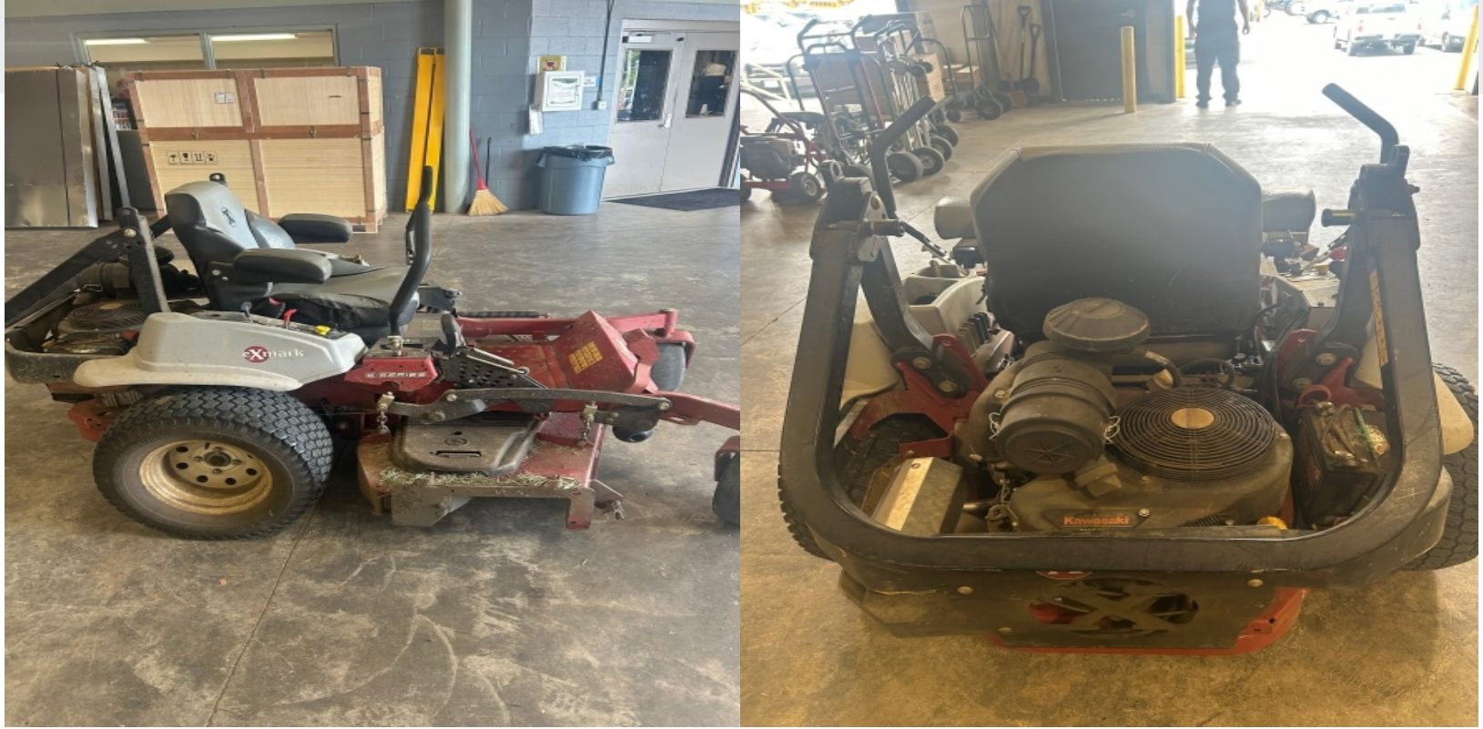
Mower #2 Laser Z E Series 60" Cut; Motor: 801V KW; Machine Hours: 910; Fair/ Good Condition; Works as should; Needs Oil Change; SN: 408687269
