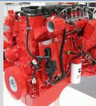
Cummings B6.7 240HP @ 560 LB FT Torque
