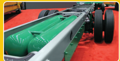
2-tank LPG system offers an estimated 300-mile range with a 70-gallon capacity.
