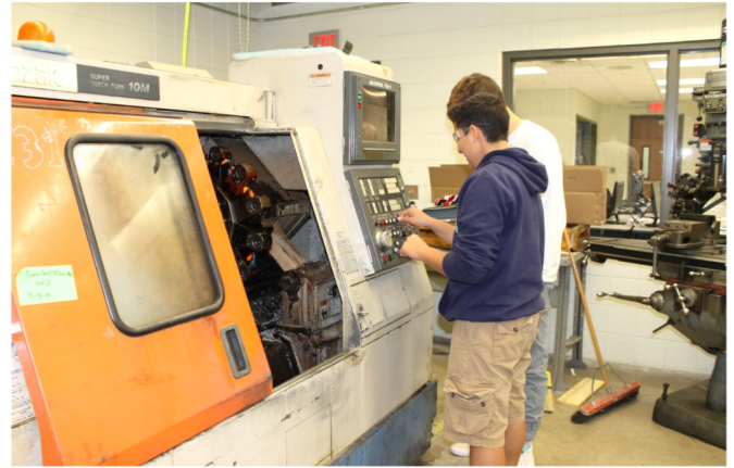
Two Rockford High School students take turns using the CNC turning center machine, which can perform various drilling operations to create cylindrical parts. This machine is valued at $20,000 and was donated to the high school’s new machine shop.
