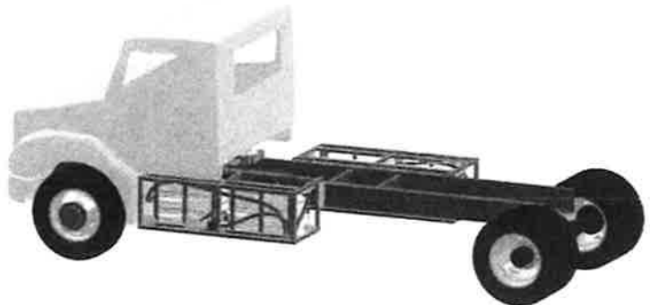
eTruck Class 6 Battery Packaging Overview
