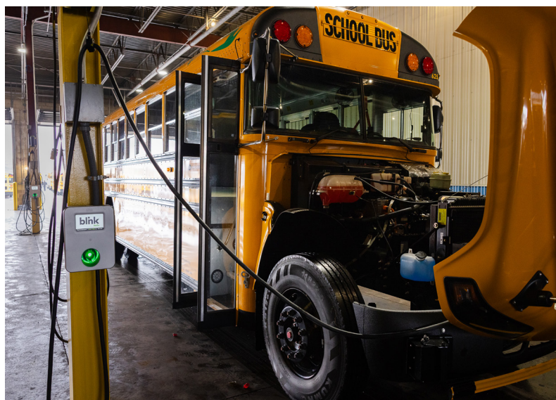
The three electric buses serving Mounds View Public Schools are charged overnight at the Northstar Bus Lines terminal in Maple Grove. Because they’re much quieter than their diesel counterparts, the buses play light music when traveling less than 15 miles-per-hour to alert nearby motorists, bikers and pedestrians.
