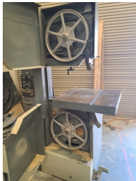
Rockwell vertical bandsaw-Bandsaw needs minor repair to drive pulley; Band welder on side does not work; Saw has been replaced with newer and smaller model
