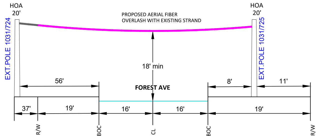
STREET CROSSING AERIAL CLEARANCE LOOKING NORTH NTS
