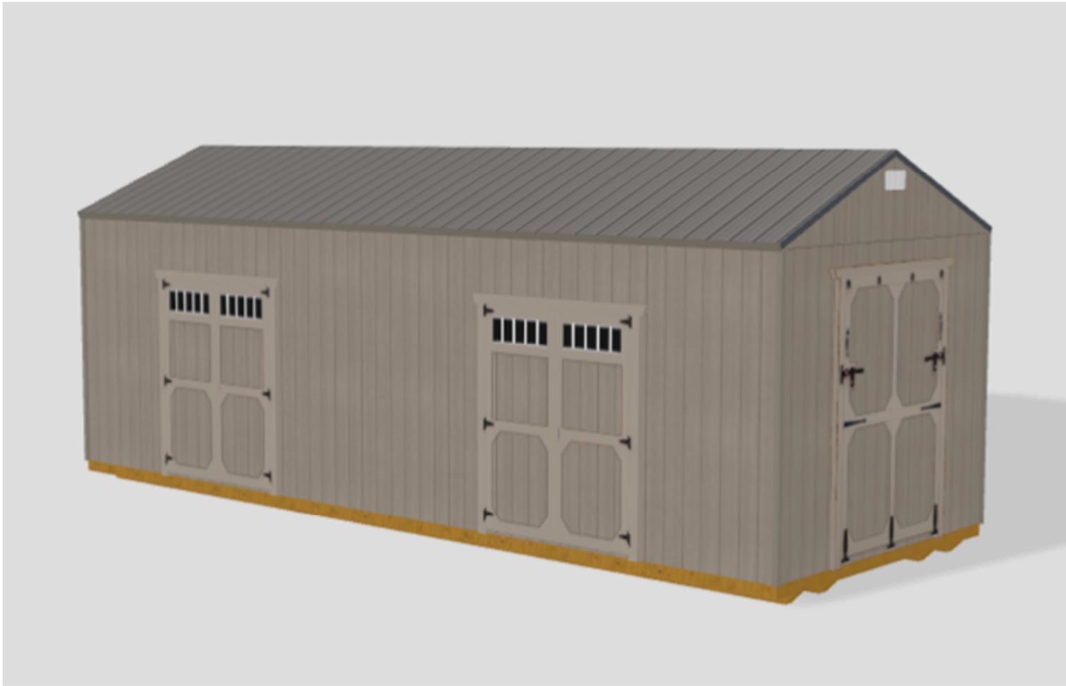
Parking lot elevation with two sets of double doors. End wall will have a ramp door that opens down to allow us to roll props in.
