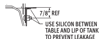
Sectional View Showing Table Connections
