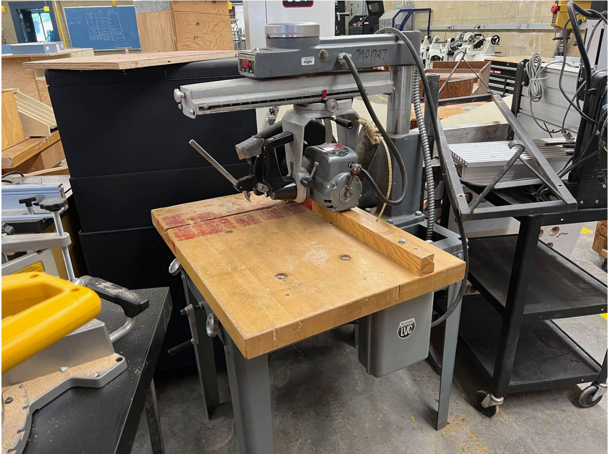
Rockwell radial arm saw. Angle adjust is stuck, however, motor runs and blade is nice as well. It does run on 220 volts.
