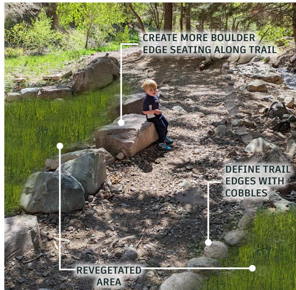
Create boulder edge seating, revegetate around trail, and define trail edges with cobbles or boulders
