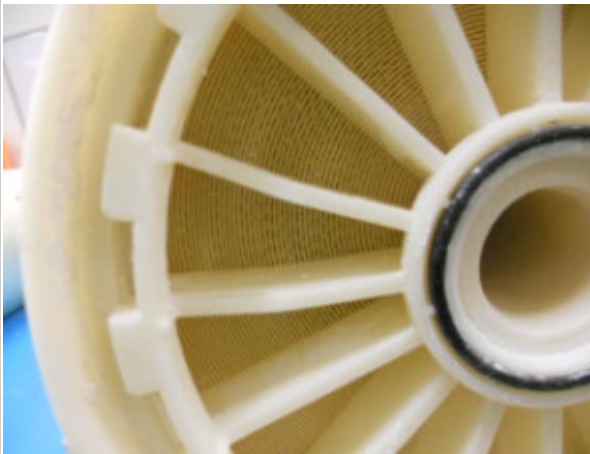
Bent spoke on the feed endcap on J4725065
