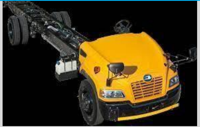
Purpose built Blue Bird OEM chassis.
