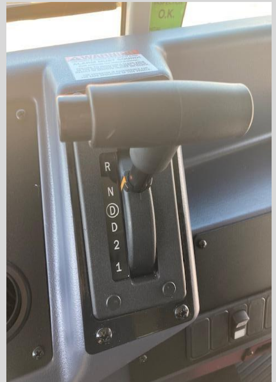
Ford 6-Speed select shift transmission.
