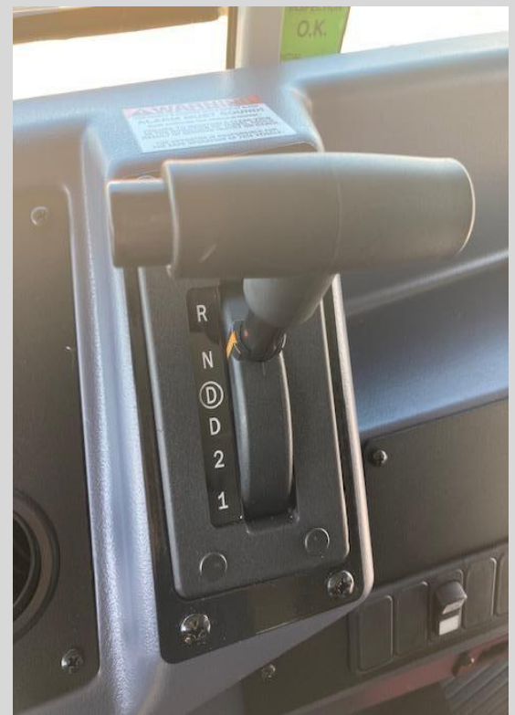
Allison 5-Speed select shift transmission.
