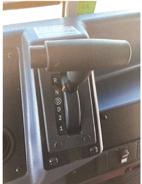
5-speed Select Shift Transmission w. cooler
