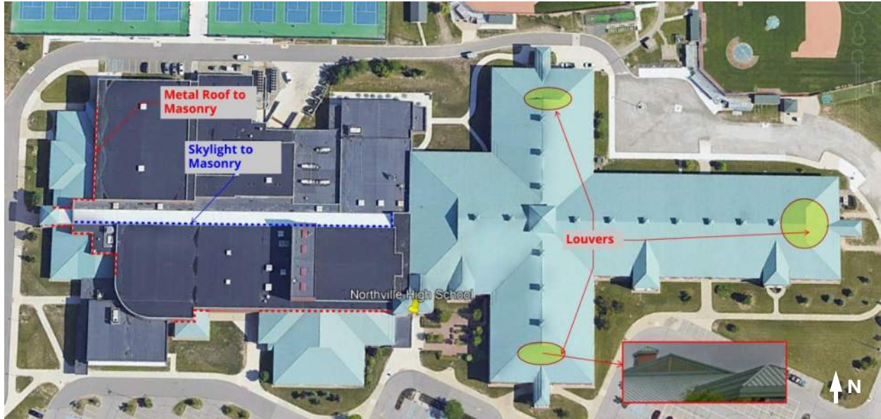
Figure 1. Annotated aerial view of the school identifying the reported regions of water infiltration.
