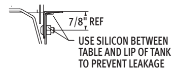
Sectional View Showing Table Connections
