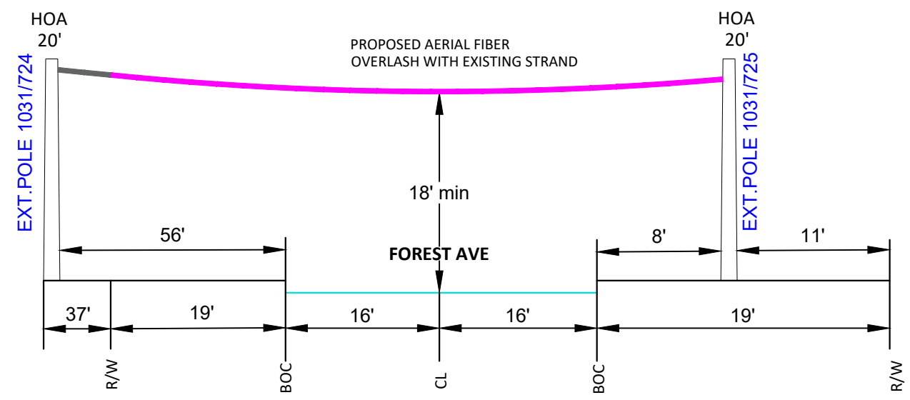
STREET CROSSING AERIAL CLEARANCE LOOKING NORTH NTS
